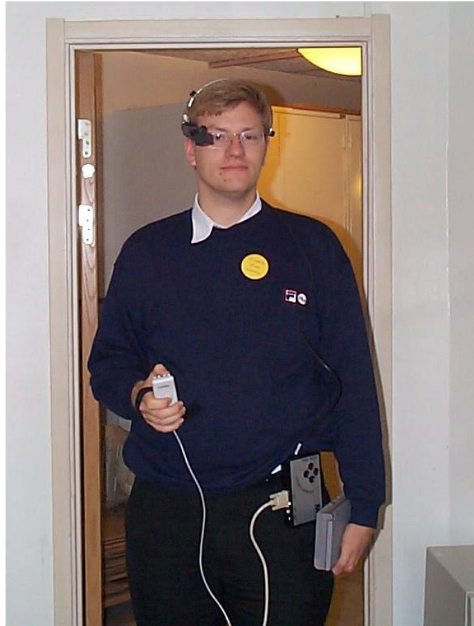
Figure 1: The author with his wearable computer, ca 1998. This includes a Private Eye 320 x 200 pixel monochrome HUD, a Twiddler one-hand chord keyboard, and a Toshiba Libretto 50 PC.
